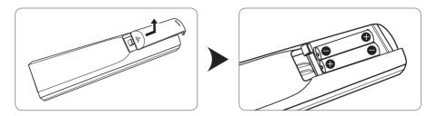
1 Remove the cover on the back of the remote control and insert the batteries.
